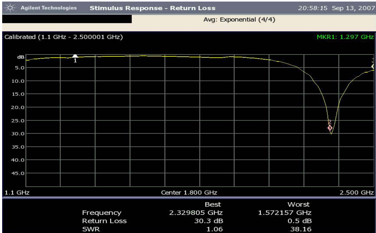
Fig. 15 Return loss for free space - 2318 MHz: 27.4dB (Marker 2)
